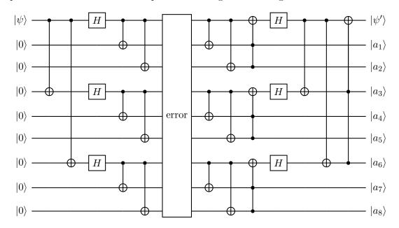
At the end of the circuit, we perform measurements on all ancilla qubits  $(|a_1\rangle, \ldots, |a_8\rangle)$  and if the measured bits are 1, we apply a NOT gate on the corresponding qubits to reset all ancilla qubits to  $|0\rangle$ .
