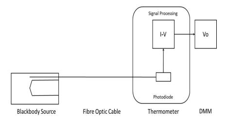
Figure 4. Configuration of laboratory testing of fiber optic thermometer.
