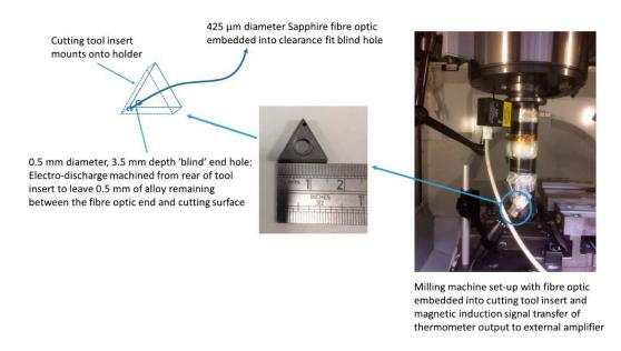
Figure 12. Milling machine set-up and schematic illustration of cutting tool insert configuration.
