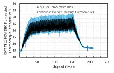
**Figure 14.** Cutting tool insert temperature measured by an embedded thermocouple from an early pass during end milling trials, illustrating broad comparability with temperatures measured by the prototype infrared thermometer.
