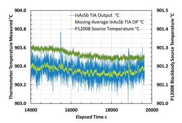
**Figure 7.** Noise in sampled thermometer signal and continuously-averaged mean thermometer signal, measuring steady-state source temperature of 900  $^{\circ}$ C.
