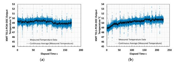
**Figure 13.** Cutting tool insert temperature recorded by fiber optic thermometer on (a) first cutting pass at minimum temperature measurable and (b) second cutting pass illustrating marginal temperature increase during milling trials.
