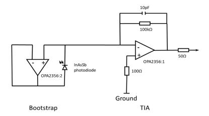
Figure 1. In AsSb photodiode bootstrapped transimpedance amplifier schematic.
