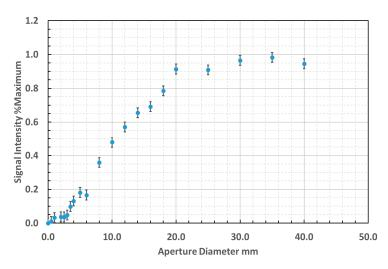
Figure 9. Field of view measurement with aperture positioned at 68 mm from fiber optic cable.
