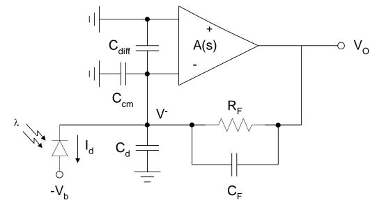
$C_s = C_d + C_{cm} + C_{diff}$   $V_O = -V^- A(s)$
