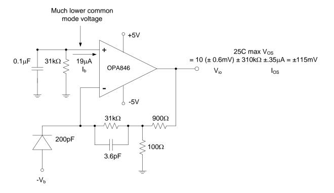
This approach does work, but will have much higher output-offset voltage than the OPA657.
