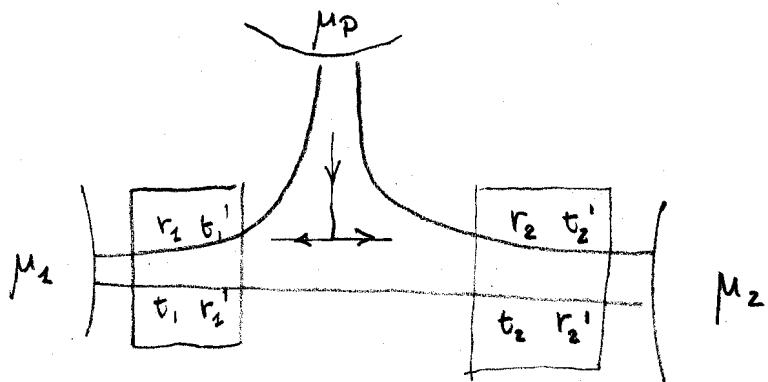
The voltage probe is at potential  $\mu_p$  and accept electrons from  $r_2$  and  $t_2$  but it also gives back them in both direction. If we just want to model dephasing without momentum relaxation we can introduce a system of twin probes like
