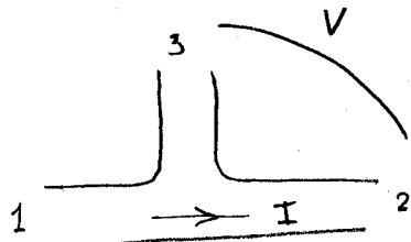
$$R_{12,32} = \frac{V_3 - V_2}{I_2} \Big|_{I_3=0}$$
