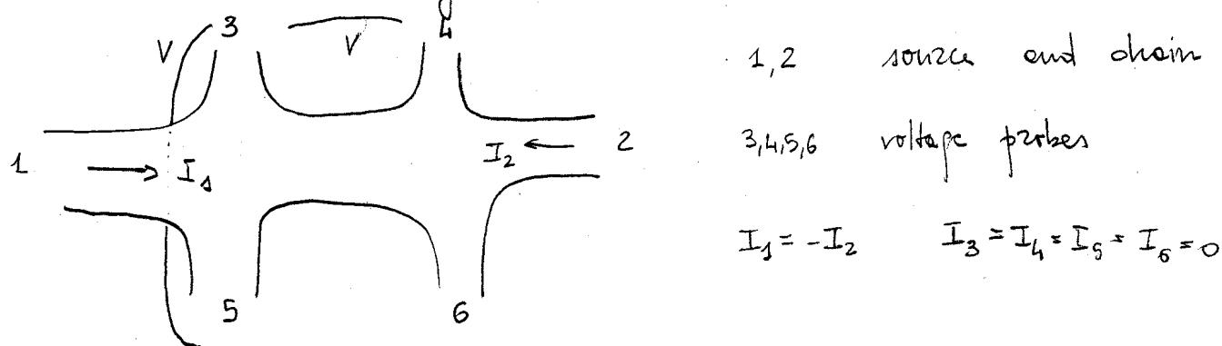
$$R_{12,12} = \frac{V_4 - V_2}{I_1}, \quad R_{12,34} = \frac{V_3 - V_4}{I_1} \quad R_{12,35} = \frac{V_3 - V_5}{I_1}$$
