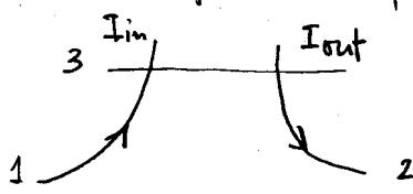
$$I_{in} = I_{out} \Rightarrow \text{no net current}$$
