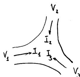
$$I_1 = G_{12} (V_1 - V_2) + G_{13} (V_1 - V_3) = (G_{12} + G_{13}) V_1 - G_{12} V_2 - G_{13} V_3$$
