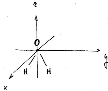
$C_2$  is a rotation of  $\pi$  around the z axis
