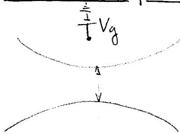
The conductance through a narrow constriction of a 2DEG (a quantum point contact) is quantized in units of  $\frac{2e^2}{h}$  where  $z$  stands for the spin degeneracy and the number of quanta depends on the width of the constriction. By modulating  $V_g$  the conductance moves in steps of  $\frac{2e^2}{h}$ .
