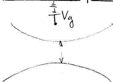
The conductance through a narrow constriction of a 2DEG (a quantum point contact) is quantized in units of  $\frac{2e^2}{h}$  where 2 stands for the spin degeneracy and the number of quanta depends on the width of the constriction. By modulating  $V_g$  the conductance moves in steps of  $\frac{2e^2}{h}$ .
